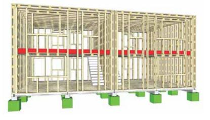
method that provides a continuous insulated seal around the core of a timber-framed structure. Using Passivhaus energy efficiency principles, the Beattie Passive system delivers a construction from foundation beams, ground floor, walls and roof all built to form a continuous void. Once in place, flame retardant insulation material is injected into the floor, wall and ceiling cavities, creating one continuous seal. Which results in no joints and no leaks.
